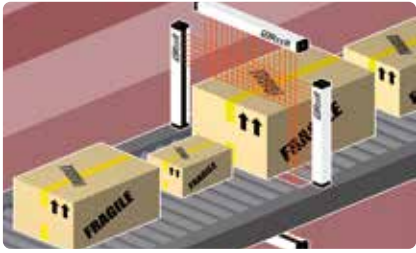
Measurement of the height of objects in transit on conveyor systems. Two-dimensional detection of objects in transit with use of 2 sets of light curtains
