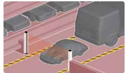
Detection of overall dimensional limits of vehicles in automated parking garages
